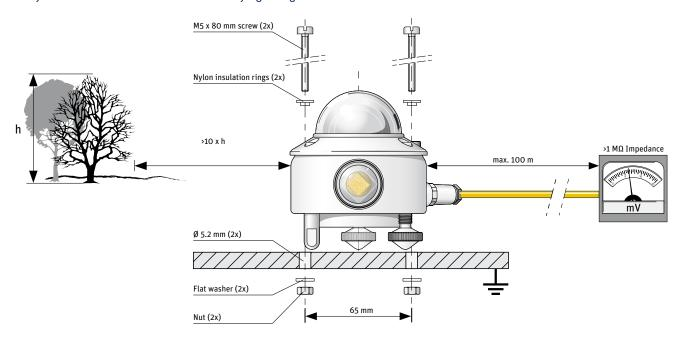
Note After recalibration and/or reinstallation ensure that the nylon insulators are refitted.
