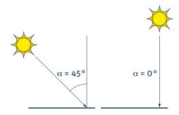
Ideally a pyranometer has a directional response which is exactly the same as the cosine-law. However, in a pyranometer the directional response is influenced by the detector and by the quality, dimensions and construction of the dome(s). The maximum deviation from the ideal cosine-response of the pyranometer is given up to 80° angle of incidence with respect to 1000 W/m² irradiance at normal incidence (0° zenith angle).
