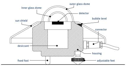
Key parts of the CMP10 pyranometer
