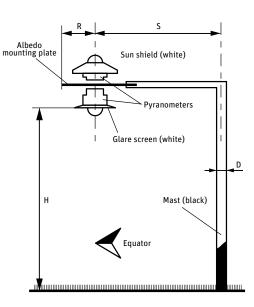
The same principles apply to the CMA 6 and CMA 11 albedometers, which already have an upper sun shield and an integrated lower glare screen and mounting rod.
