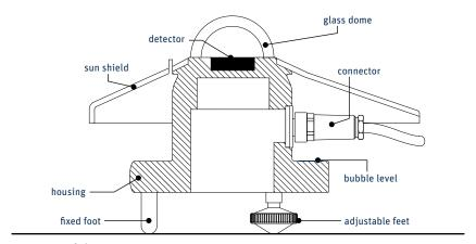
Key parts of the CMP 3 pyranometer
