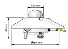
CMP 6, CMP10, CMP 11, CMP 21 and CMP 22 Weight without cable: 0.6 kg
